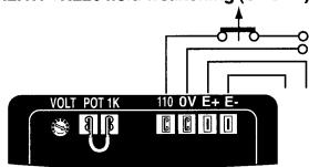
The exciter is switched off by disconnecting the AVR power supply (1 wire - 0 or 110V). Contact rating: 16A - 250V alt.
